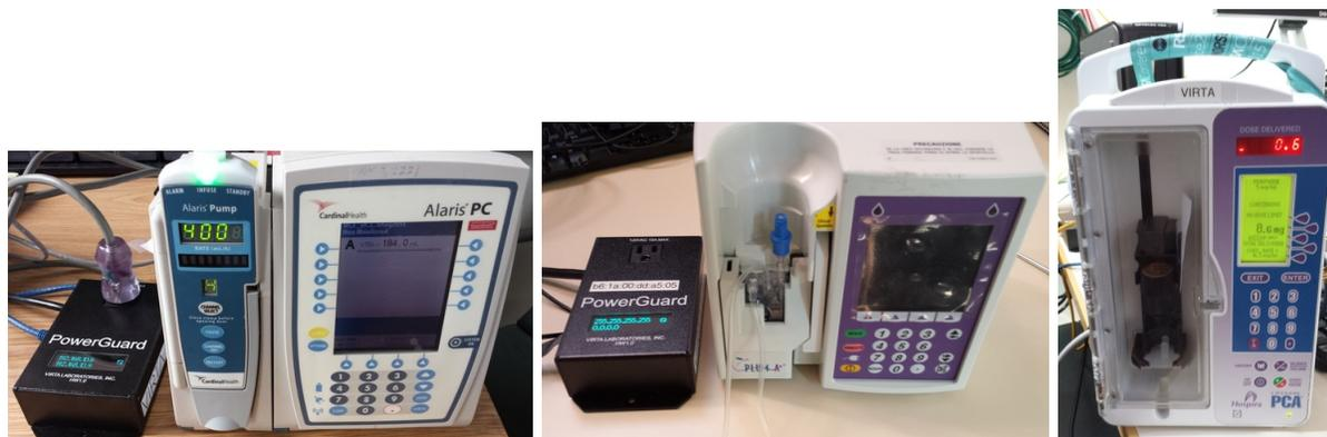
Figure 1: Photos of infusion pumps tested. Left: Alaris 8100 Large Volume pump with an Alaris 8015 PC unit. Center: Hospira Plum A+ large-volume pump, infusion bag type. Right: Hospira Lifecare PCA, syringe type. Also shown: PowerGuard™ pass-through power outlet.
