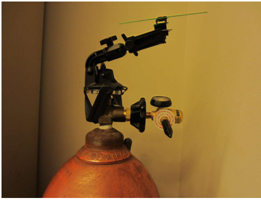
Fig. 11. The WISPCam , mounted on an industrial gas cylinder, monitors a pressure gauge.
